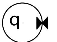
$$q = k \sqrt{\Delta p_m} \quad (\text{l/s}) \quad (\text{Pa})$$
