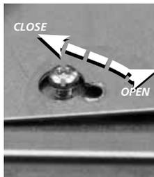
The fan is easy to open for cleaning and service with the swing-out design. Loosen the screws a few turns, without removing them. Turn the motor bracket to the right so the screws can go through the key holes. Open the motor bracket. When closing, turn the motor bracket to the left so the screws go into the smaller part of the keyholes. Tighten the screws.
