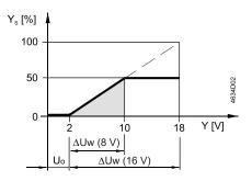
Max. positioning range Ysmax = 100 % (90°) Span Ys = 50 % (45°) Offset Uo = 2 V Virtual span  $\Delta$ U = 16 V Effective span  $\Delta$ U = 8 V
