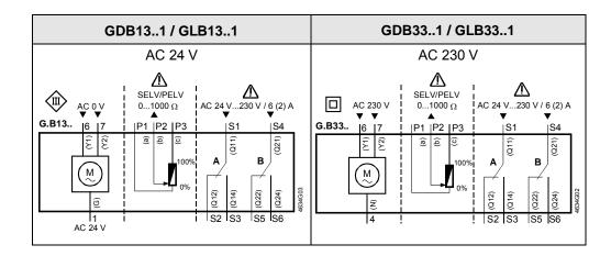
Modulating control Y = DC 0...10 V, 0...35 V
