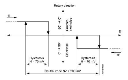
The diagram shows the relationship between the differential voltage E = Y - U (difference between setpoint Y and actual value U) and the rotary direction, including hysteresis and neutral zone.
