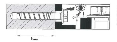
Ensure that the screw anchor head fully rests without any gap on the fixture and is not damaged
